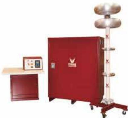
AC, Tank Type, 300 kV, 150 kVA
