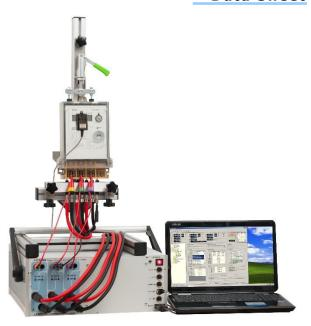
The Calmet TB10 Test Bench employs modern precision power source with the internal reference (without need to use an additional external reference energy meter with additional cables). By this conception may be achieved simultaneously flexible customer orientated solution characterised by extremely compact size, light weight, high metrological properties at reasonable price.
